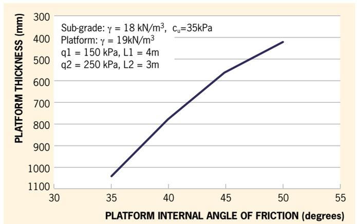
Figure 1: Platform thickness v internal angle of friction
