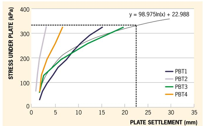
Figure 4: Plate bearing tests on loose granular sub grade
