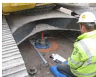
Set up for plate bearing test
