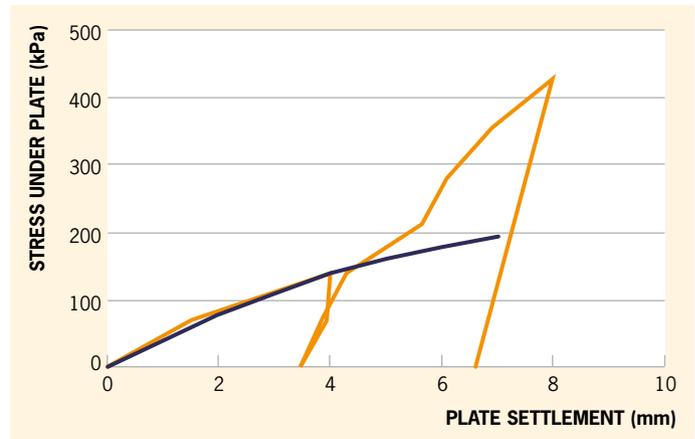
Figure 5: Plate bearing tests on uncompacted platform
