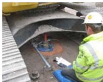
Set up for plate bearing test
