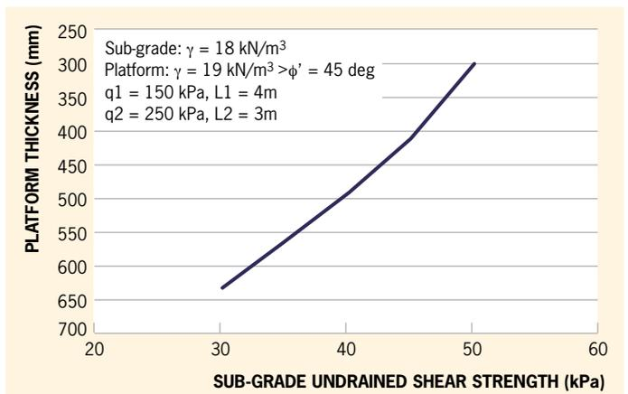
Figure 2 Platform thickness v sub-grade undrained shear strength
