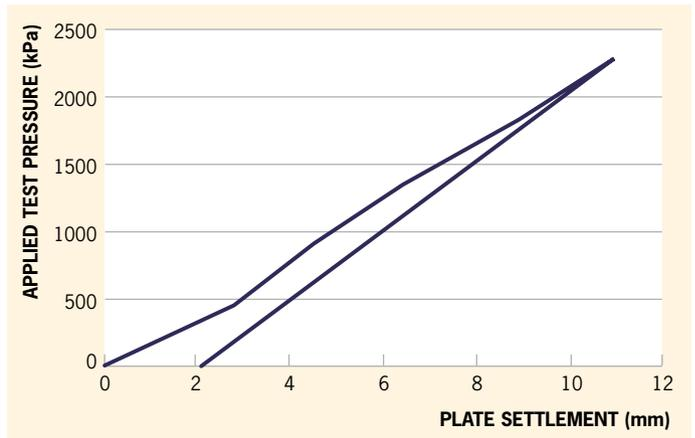
Figure 3: Working platform material plate loading test
