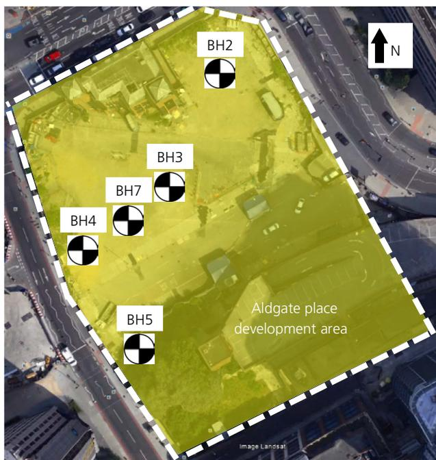
Figure 3. Site investigation borehole layout plan
