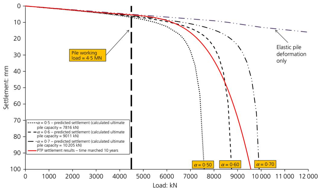
Figure 6. Loadtest-predicted settlement under load with London Clay adhesion factor ( $\alpha$ ) varied and PTP settlement data time-marched 10 years
