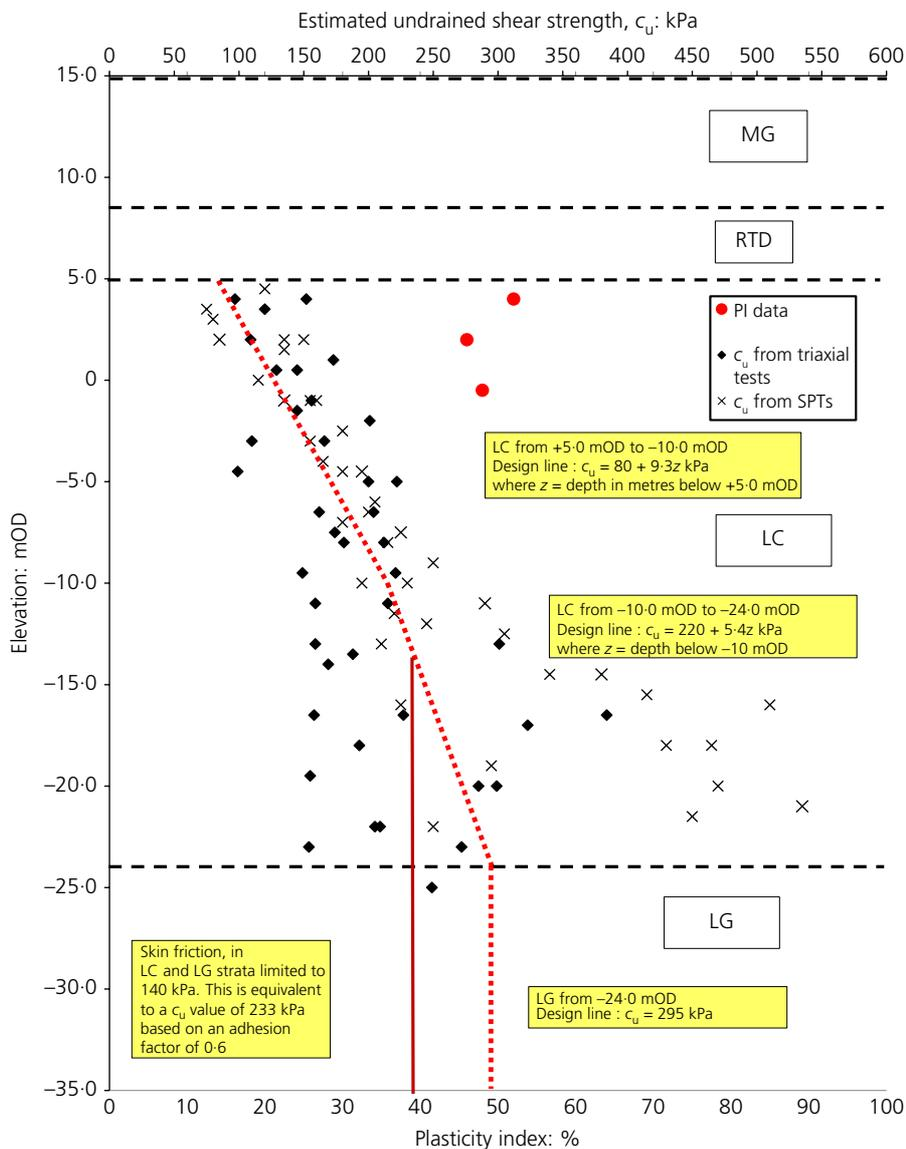
Figure 5. Undrained shear strength ( $c_u$ ) and plasticity index (PI) plotted against elevation and the proposed design line
